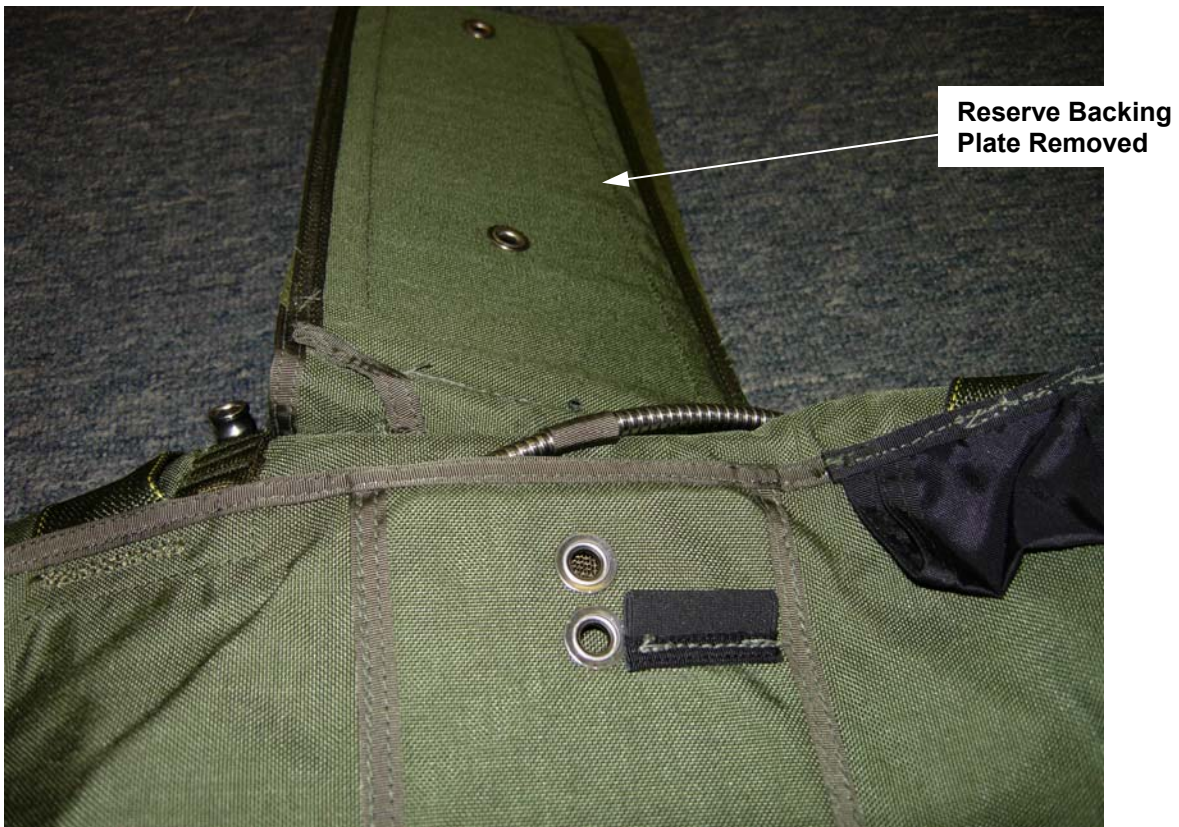
Figure 1. Harness/Container With Reserve Backing Plate Removed.
