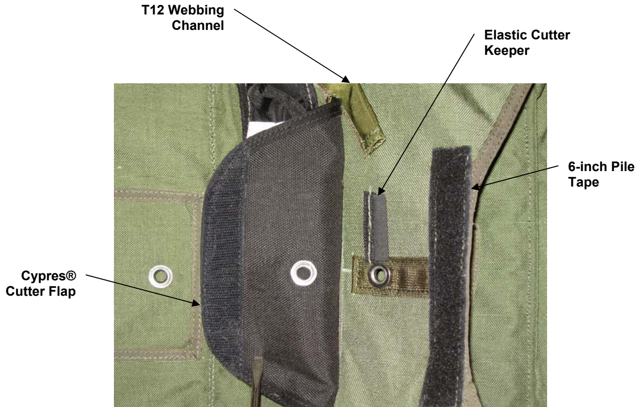
Figure 4. Harness/Container With Modification, View 3.
